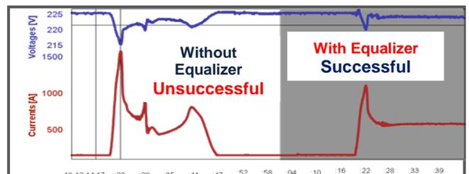
As a centralized compensation solution, Equalizer design provides the reactive current requirements for several motors, saving on additional devices on a multi-motor site. The Equalizer accommodates both low and medium voltage installations. Due to the short time reactive energy requirements, the size of the step up transformer is minimized making the Elspec Equalizer an extremely **cost effective** solution.
